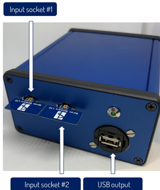
Figure 2: Driving circuit box with two sensors connected.
